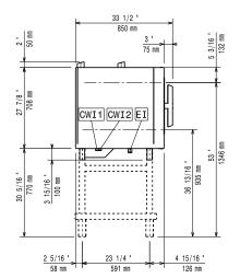
Cold Water inlet 1 (cleaning) Cold Water Inlet 2 (steam CWII CWI2
